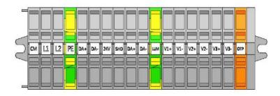
The NES-1K8T210BC supports a 'common anode' (common Vo+) connection.
