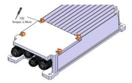
Section 2. Assemble cable on the driver
